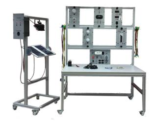
Solar energy is renewable energy type which is an important subject in the world today. This is a modular type experiment set. The location of the modules can be changed. With safe electrical cables these modules are connected. The system is used for demonstrate of a photovoltaic system with grid connected operation with inverter by utilising electrical components from the real world usage of photovoltaics.
